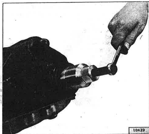
FIG. 205—PULLING OUTPUT SHAFT OIL SEAL
