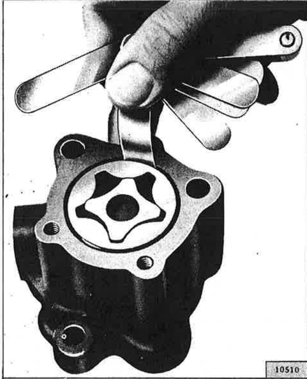
FIG. 55—CHECKING OUTER ROTOR TO OIL PUMP BODY
